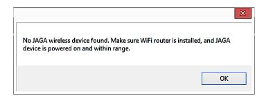
**Solution 1:** Once you powered the JAGA device with a battery, Make sure you first see red blinking LED for a few seconds on the JAGA16 device and disappears *before* you click **Start display** in NeuroPhys.
